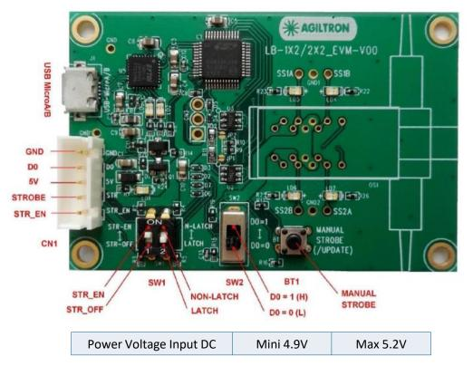
The two configuration switches S1 and S2 are present to match switch type. Do not change it.
