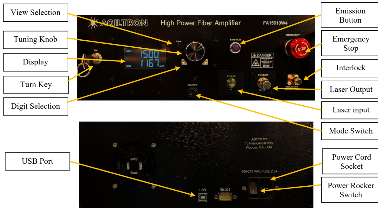
Figure 2: Front and rear panels of amplifier.
